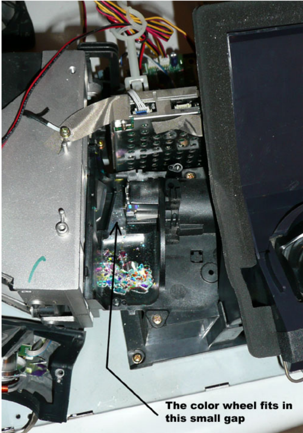
Color wheel housing interior shown much larger than life.
